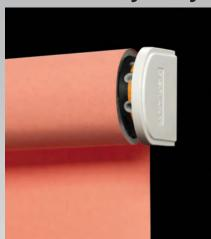
Features: Heavy-duty white plastic covered / metal brackets for face or top fixing, with 53 or 60mm grooved aluminium barrel. Fabric is located in the groove in such a way that, although it cannot be pulled out it may be slid out sideways for repair or replacement. A powerful 240v AC motor is housed within the barrel and is operated by an individual switch. Tear Drop white aluminium bottom bar as standard.
