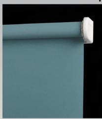
**Features:** White plastic brackets with 23, 32 or 36mm aluminium barrel housing a premium quality spring with decelerator mechanism. The rigid white plastic bottom bar is fabric covered at front and has a central cord-pull.
