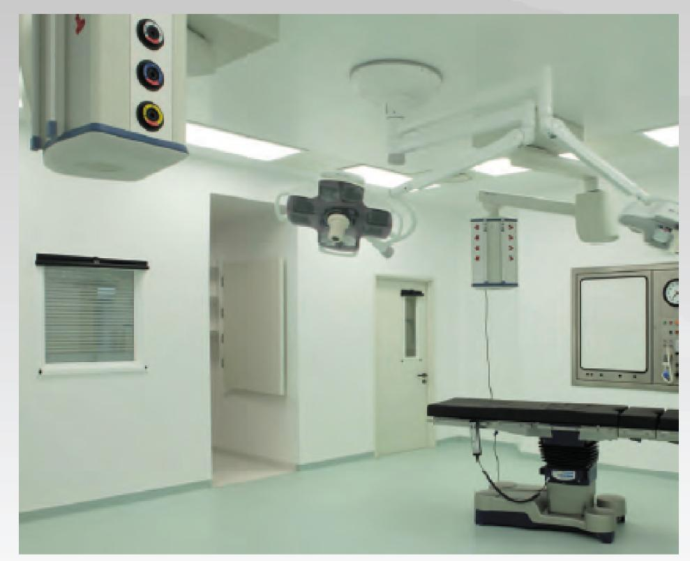
Features: Laser Material to protect from Stray Laser Radiation is available on all SK roller blinds. Designed to use as passive guards where Class 3B or Class 4 lasers are in use. All material is certified to EN 60824 -4 (Safety of Laser Products Part 4: Laser Guards) and is fire proof.
