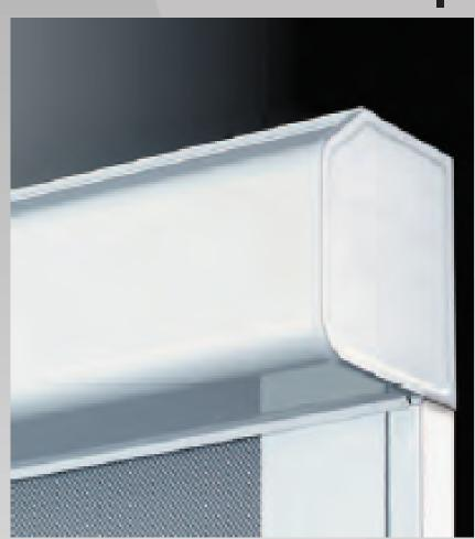
Features: C65-85: Aluminium cassette 85 x 97mm with metal end plated and top-fix or face-fix brackets. A heavy duty 240v motor housed within a 53mm barrel to which the fabric is attached. The motor is controlled by a switch which may be surface or flush mounted. Fabric has a 12 x 42mm bottom bar, running in 55mm side channels. Studs fitted at edge of fabric to retain it within side channels. Black or white hardware as standard. C65-115: As C65-85 apart from: cassette size115 x 132mm.
